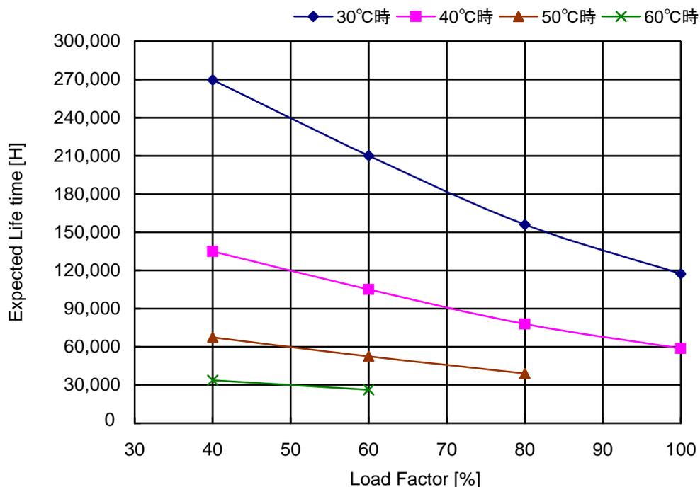
Over the area of 15 years, the degradation of sealing rubber, etc., is not included in the calculation
