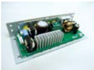
Trial PSU developed by junior engineers Single output general purpose PSU
