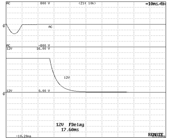
Output Fall Characteristics (magnification)
