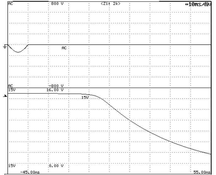
Output Fall Characteristics (magnification)
